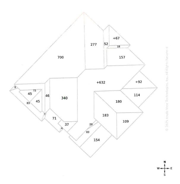
Note: This diagram shows the square feet of each roof facet (rounded to the nearest Foot). The total area in square feet, at the top of this page, is based on the non-rounded values of each roof facet (rounded to the nearest square foot after being totaled).
